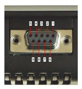
Figure 6: Pin assignment RS-232 (D-Sub 9-pole female)
