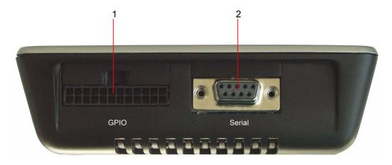
Figure 1: TC65 Terminal front view
