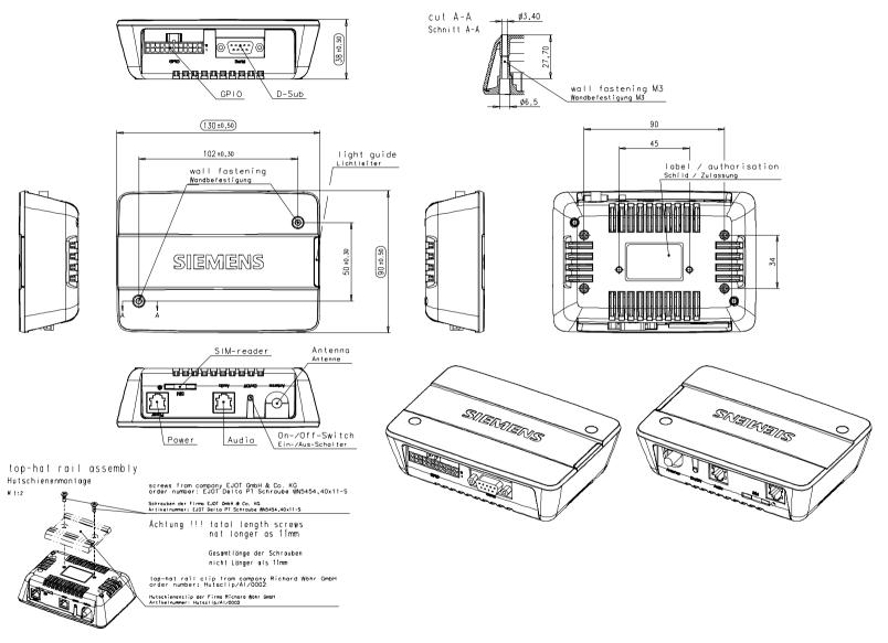
Figure 13: Mechanical dimensions
