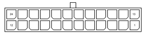
Figure 10: IO interface connector front view
