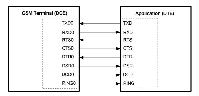
TC65 Terminal is designed for use as a DCE. Based on the conventions for DCE-DTE connections it communicates with the customer application (DTE) using the following signals:
