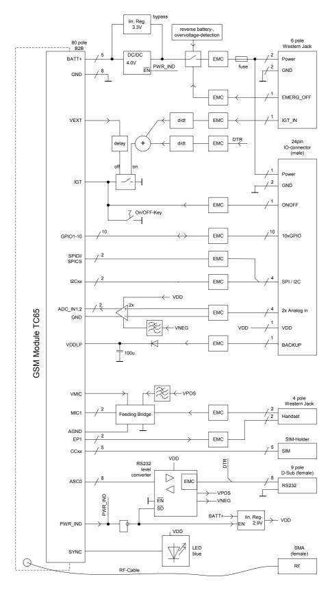
Figure 4: TC65 Terminal circuit block diagram
