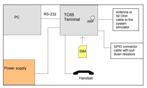
Figure 18: Reference equipment for approval
