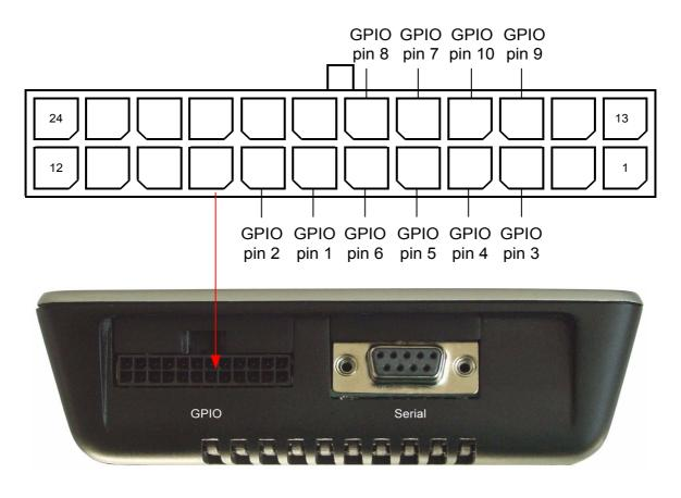
Figure 11: Location of GPIO pins
