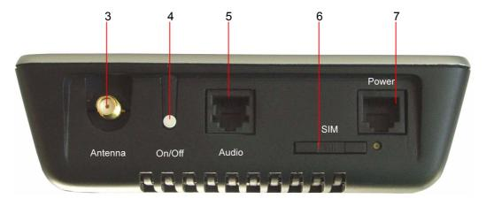
Figure 2: TC65 Terminal rear view
