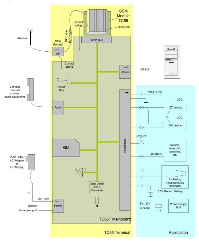
1) Fast acting fuse 1,25A , (0.9...1.3  $\mbox{A}^2\mbox{s}$ ) is recommended for 24V vehicle supply only.
