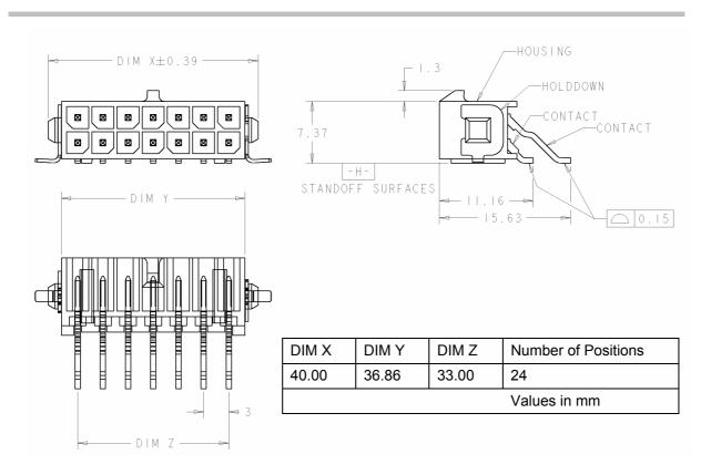
Figure 17: Mechanical dimensions of the Tyco Mate\_N\_LOK connector on the TC65 Terminal.
