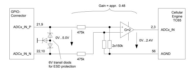
Figure 12: ADC balanced amplifier
