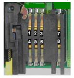
Figure 9: Pin location of the Molex SIM card holder and position
